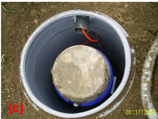
Figure-4: Photographs of NISN stations (a) KSSS and (b) KESM. Buried in the ground and protected by separate plastic barrels are the (c) the STS-2 sitting on a concrete pier cemented to the bedrock and temperature insulated by a thermos, and (d) the Q330 digitizer, Baler, power controller and battery.
