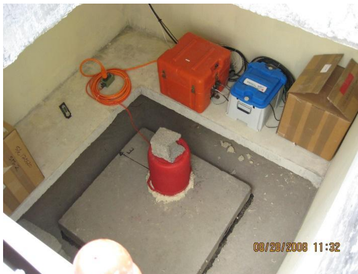
Figure-7: Photograph showing the inside of a KSIRS underground concrete vault with the data acquisition and power systems are placed on the built-in shelf. The seismometer is sitting on the pier and covered by an inverted thermos to minimize the effect of temperature variation.
