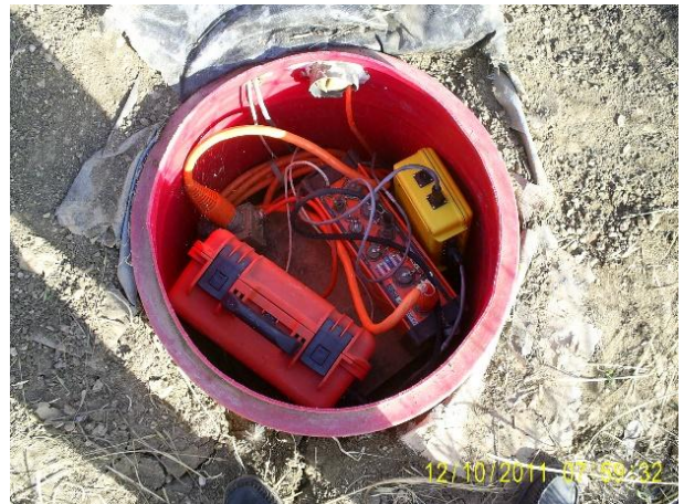
Figure-4: Photographs of NISN stations (a) KSSS and (b) KESM. Buried in the ground and protected by separate plastic barrels are the (c) the STS-2 sitting on a concrete pier cemented to the bedrock and temperature insulated by a thermos, and (d) the Q330 digitizer, Baler, power controller and battery.
